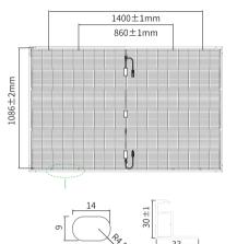
Noted: For specific dimensions and tolerance ranges, please refer to the corresponding detailed module drawings.
