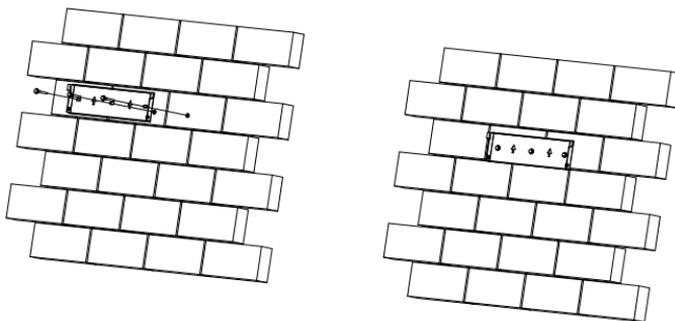
Figure 4.8 Mount the rear panel of R5-0.7K-3K-S1 & R5-3K-8K-S2
