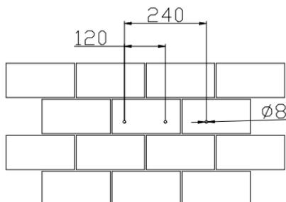
Figure 4.7 Drill holes' dimensions of R5-3K/3.6K/4K/5K/6K/7K/8K-S2
