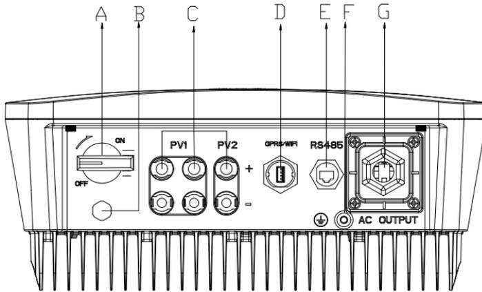
Figure 5.3 Electrical interface of R5-7K/8K-S2
