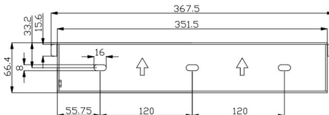
Figure 4.5 Dimensions of rear panel of R5-7K/8K-S2
