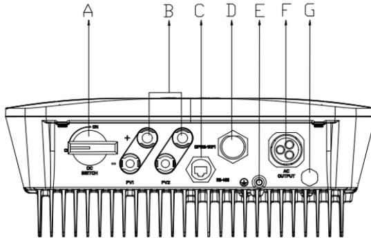
Figure 5.2 Electrical interface of R5-3K/3.6K/4K/5K/6K-S2
