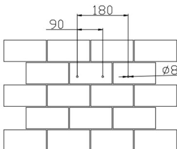
Figure 4.6 Drill holes' dimensions of R5-0.7K/1K/1.5K/2K/2.5K/3K-S1
