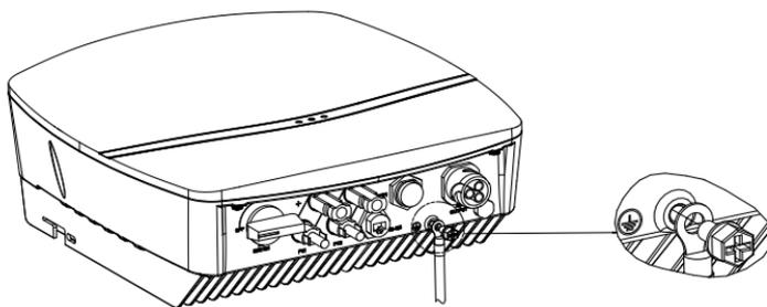
Fig. 5.4 Inverter ground protection
