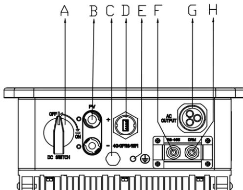
Figure 5.1 Electrical interface of R5-0.7K/1K/1.5K/2K/2.5K/3K-S1
