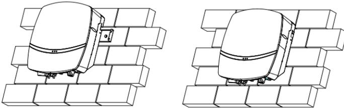
Figure 4.9 Mount R5-0.7K-3K-S1 & R5-3K-8K-S2 inverter
