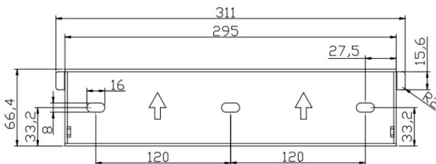
Figure 4.4 Dimensions of rear panel of R5-3K/3.6K/4K/5K/6K-S2
