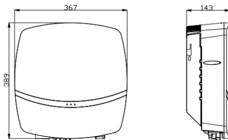
Figure 3.3 Dimensions of R5-3K/3.6K/4K/5K/6K-S2
